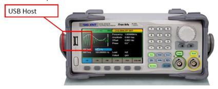
2. Press the Utility key on the front panel, and then softkey "System ->Page 1/2 -> Firmware Update", to enter the interface of the file browser.
