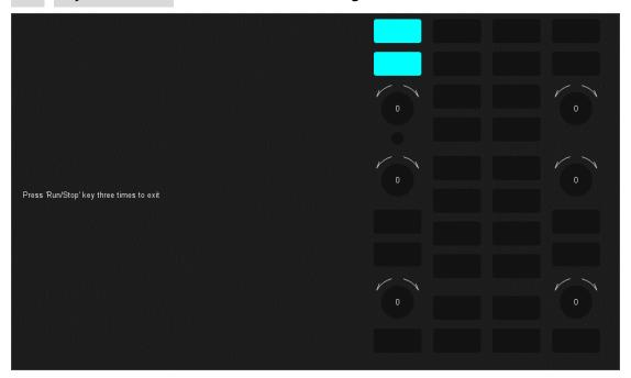
**Knob test:** Turn each knob clockwise, counter-clockwise, and press down. Observe whether the value on the corresponding knob (default 0) on the screen increases or decreases in real-time and whether the knob lights up when it is pressed.
