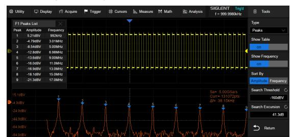
The following shows the peak tool enabled for an FFT waveform:
