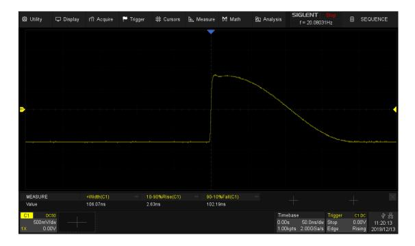
In the example, 5000 pulses can be obtained with the sample rate of 2 GSa/s at the maximum memory depth.
