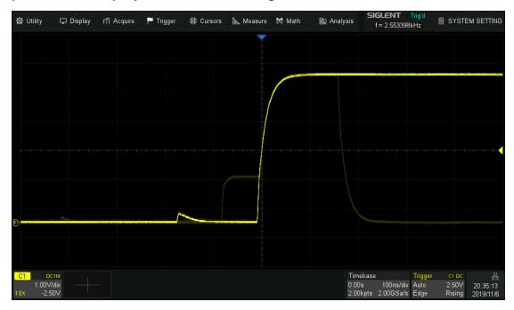
In this case, the zone trigger is a quick and simple way to capture the interesting waveform. Enable the zone trigger, and draw a box to intersect with the bus contention part, as shown in the figure below:
