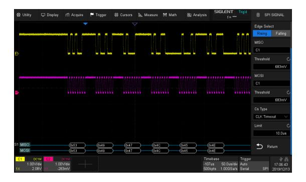
If the data width is set to be greater than 8-bits (such as 16-bits), measure the clock idle time between 8-bit data packets as 20  $\mu$ s, and then set the timeout time to a value between 20 and 300  $\mu$ s. In this example, it is set to 30  $\mu$ s:
