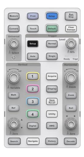
The front panel is designed to operate the basic functins without having to open the software menu. Most of the front panel controls duplicate functionality available through the touch screen display but the operation is more quickly achieved.
