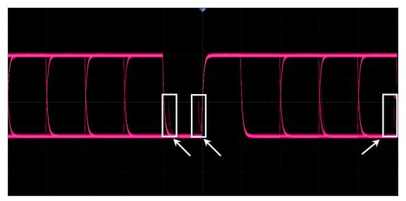
When the display dialog box and persist are off, double-pressing the Display/Persist button on the front panel can quickly turn on persistence.
