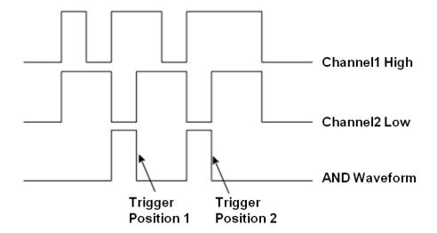
Logic (AND, OR, NAND, NOR), source, limit range, and time value can be set in the trigger dialog box. When the logic is "OR" or "NAND", the setting of the time limit is invalid.
