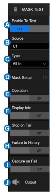
When it is "on", the failure waveform is detected, the screenshot with failure frame will be stored in the external U disk.
