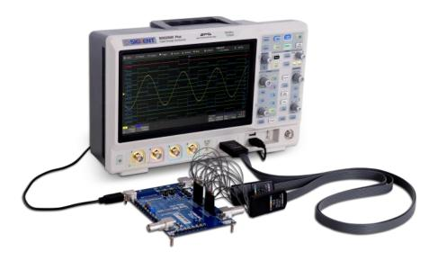
**To connect the logic probe:** Insert the probe, with the correct side facing up, until you hear a "click".
