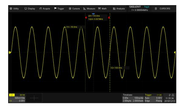
Fixed delay, timebase is changed to 100 ns/div, the value of X cursors (-50 ns, 100 ns) remains fixed. The grid number of X cursors are changed to -0.5 div, 1 div.
