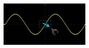
Draw a rectangular box to create a zone or a histogram region. At the beginning of the gesture keep the angle close to 45°so it can be recognized as the drawing box gesture
