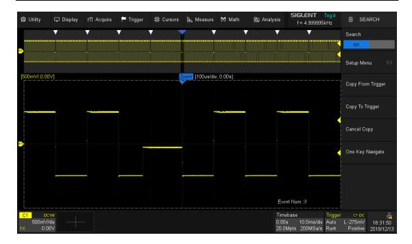
Press the Run/Stop button on the front panel to stop the acquisition, and then follow the steps Navigate Type to select "Search Event". The following figure shows the first dwarf pulse. In this example, the list is enabled and time labels of each event are shown in the list.
