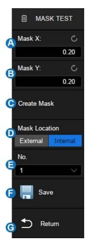
Set the values for  $Mask\ X$  and  $Mask\ Y$  (in divisions of display graticule), and then perform  $Create\ Mask$  to generate the mask. The horizontal and vertical adjustment range is  $0.08{\sim}4.00$  div.
