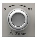
When the Zoom function is on, the waveform area is divided into upper and lower parts. The area of about 1/3 height above is the main window, and the area of about 2/3 height below is the zoom window. Touch a window to activate it.
