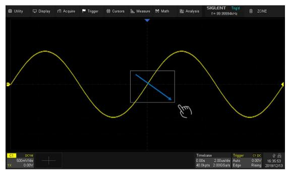
When the finger moves out of the screen, a menu pops up for selecting the zone and setting the zone properties:
