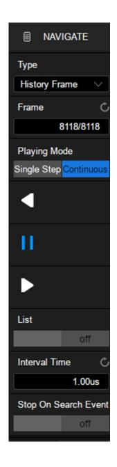
Touch *Interval Time* to set the playing interval by the universal knob or the virtual keypad.
