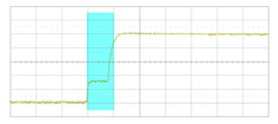
With a simple edge trigger, it is unlikely to trigger consistently on this
