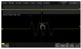
Adjust the horizontal position of the zoom area by dragging left and right in the zoom area of the main window or waveform in Zoom window
