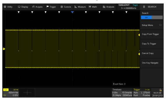
Turn on Zoom function to observe the full view of the frame and the detail of the third dwarf pulse at the same time:
