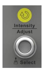
When the parameter setting area is highlighted, you can use the Universal Knob to adjust or set the parameter. Press the knob to select an option from the list. The default function of the Universal Knob is to adjust the intensity of the waveform traces.
