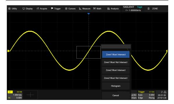
Once a zone is created, it can be moved by dragging. Just touch and hold the zone box and use a dragging gesture.
