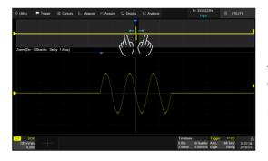
Adjust the horizontal scale of the main window by pinch and spread in the gray area of the main window
