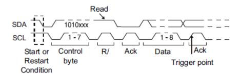
**7 Address & Data** — the oscilloscope will be triggered on read or write frame in 7-bit address mode.
