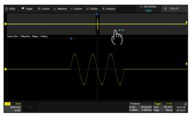
Adjust the horizontal position of the waveform by dragging left and right in the gray area of the main window
