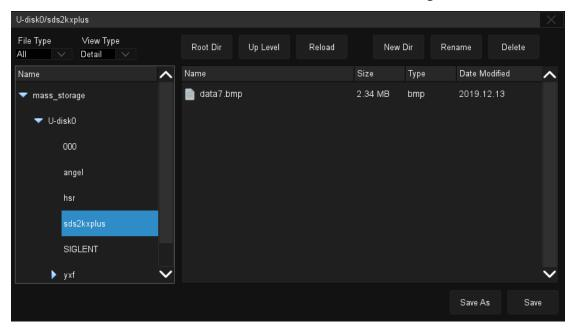
In step 4, if Save is selected instead of Save As, the system saves the file as the default file name sds2000X Plus\_BMP\_n.bmp, where n is an integer incrementing from 1. The default save path is \SIGLENT\.
