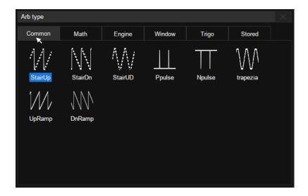
There are 6 tabs in the window. Under each tab, a catalog of waveforms are listed. Built-in waveforms are stored in Common, Math, Engine, Window, and Trigo. Stored waveforms are located in the Stored menu.
