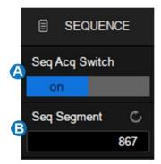
Sequence mode is a fast acquisition mode, which divides the memory depth to multiple segments (up to 90,000), each of which stores a single shot. In sequence mode, the oscilloscope only acquires and stores data without processing and displaying, until the specified segments are acquired. As a result, the dead time between trigger events is minimized, thus greatly improving the waveform update rate. If sequence mode is
