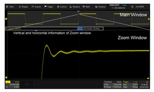
The area not covered by the gray background in the main waveform area is the region to be zoomed in (zoom area). When the zoom window is activated, the zoom area can be expanded or compressed by rotating the horizontal and vertical scale knob. Rotating the horizontal and vertical position knob to move the position of the region. When the main window is activated, the scale knobs and position knobs are used to change the
