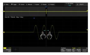
Adjust the horizontal scale of the Zoom window by horizontal pinch and spread in the zoom area of the main window or in the Zoom window
