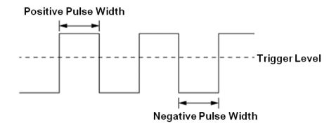
**Less than a time value (≤)** -- Trigger when the positive or negative pulse time of the input signal is lower than the specified time value. Below is an example of trigger condition is set to positive pulse width < 100ns
