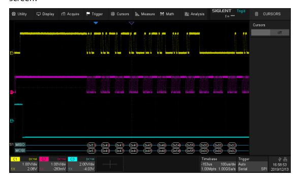
When the CS type is set to Clock Timeout, turn on Cursor, measure the clock idle time between frames as 300  $\mu$ s, and measure the interval between clock pulses as 2.4  $\mu$ s, then set the timeout to a value between 2.4 and 300  $\mu$ s. In this example it is set to 10  $\mu$ s:
