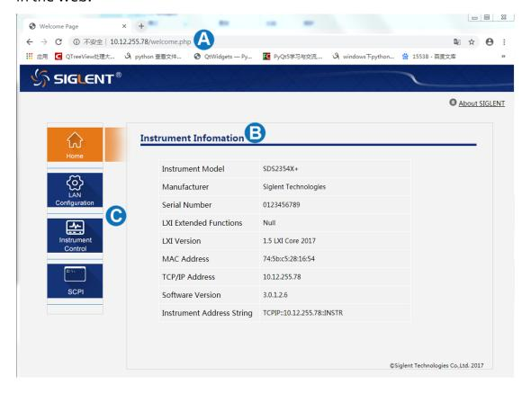
A. Input the IP address of the instrument
