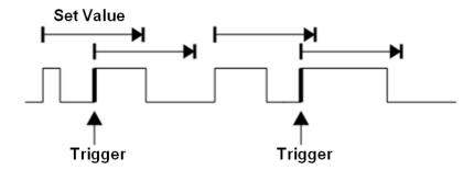
Trigger source, slope (rising, falling), limit range and time value can be set in the trigger dialog box. Holdoff, coupling, and noise reject can be set in the interval trigger, see the sections "Holdoff", "Trigger Coupling" and "Noise Reject" for details.
