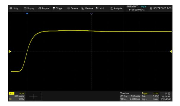
Fixed delay, timebase is changed to 5 ns/div, the horizontal delay value remains fixed, while the grid number of delay changes to -4 div
