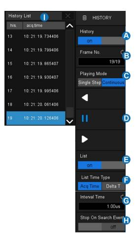
The oscilloscope automatically stores acquired frames. It can stores up to 90,000 frames but the number may vary due to the memory depth and timebase settings. Turn on history mode, then the stored frames can be
