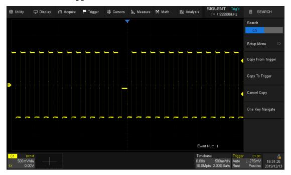
Then turn on the Search function and operate *Copy from Trigger* in the search dialog box so that the oscilloscope searches for the dwarf pulses according to the same setting as the trigger.
