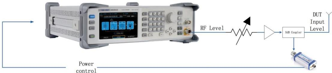
As shown in the example, the sensor measures a proportional power in defined time intervals, derived from a coupler. It considers optionally the given S-parameters and returns the results to the generator. The signal generator compares the measured level with the set value and adjusts its output level accordingly. This allows you to control the external signal level continuously and reliably reach a constant input level at the DUT in real time.
