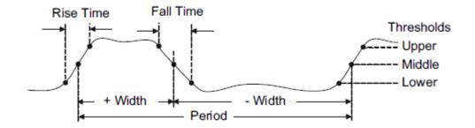
Figure 89 Time Measurements
