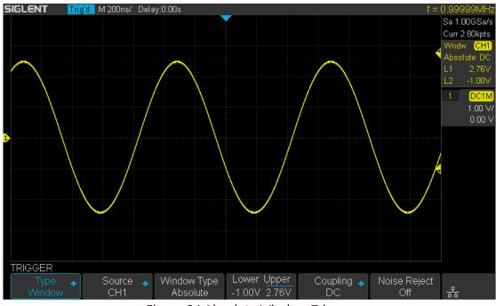
Figure 34 Absolute Window Trigger
