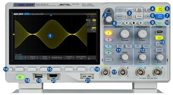
Figure 9 SDS1000X-E 4-Channel Scope Front Panel Overview
