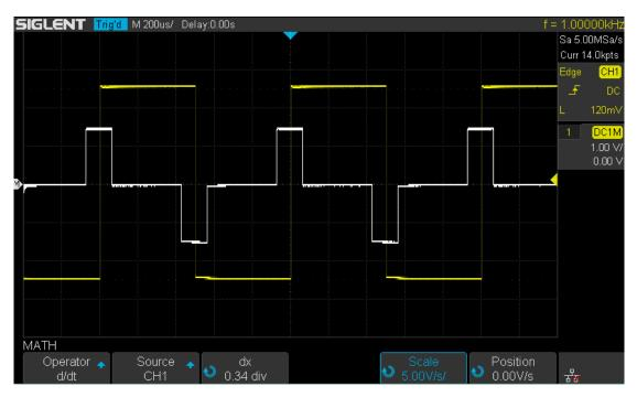
Figure 81 Difference Function Operation
