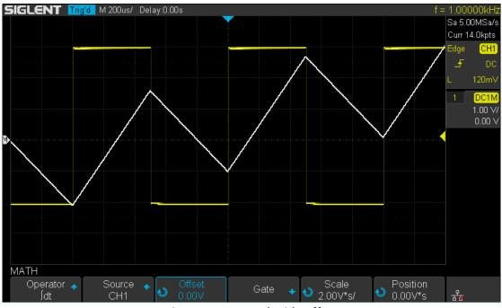
Figure 83 Integral with Offset
