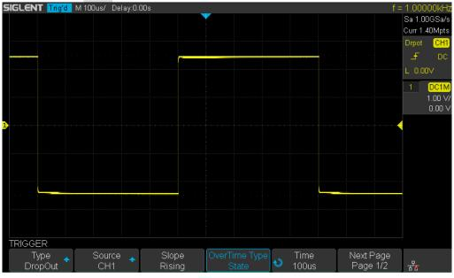
Figure 38 State Dropout Trigger
