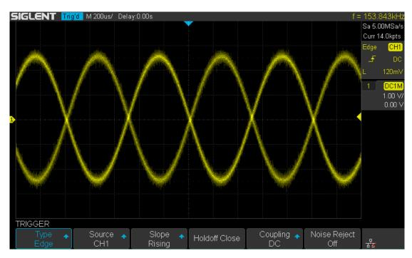
Figure 28 Turn off the Noise Reject
