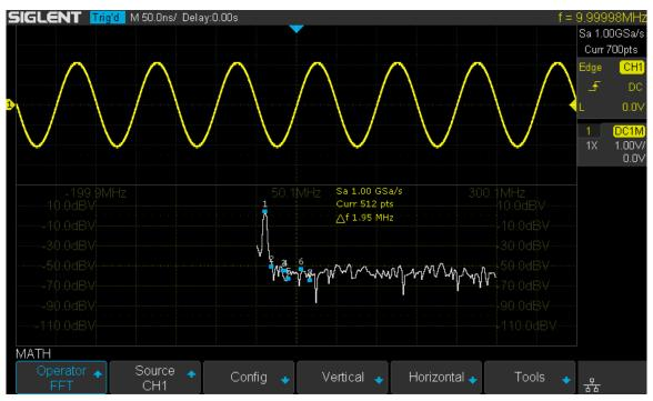
Figure 80 FFT Waveform
