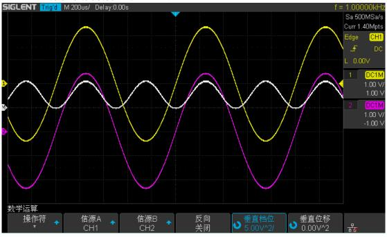
Figure 71 C1\*C2 Waveform
