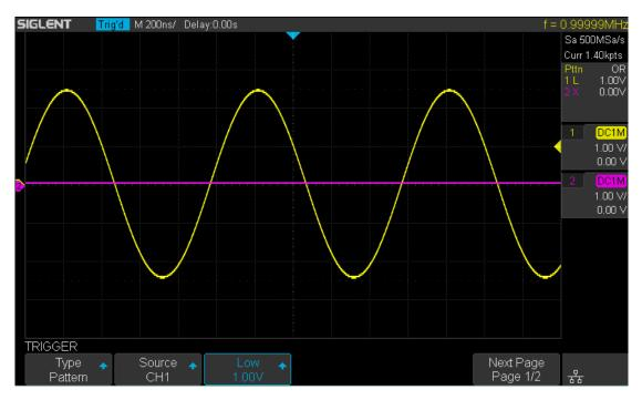
Figure 40 Pattern Trigger
