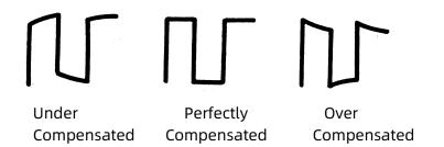
4. Use a nonmetallic driver to adjust the low-frequency compensation adjustment hole on the probe until the waveform displayed is as the "Perfectly compensated" in the figure above.
