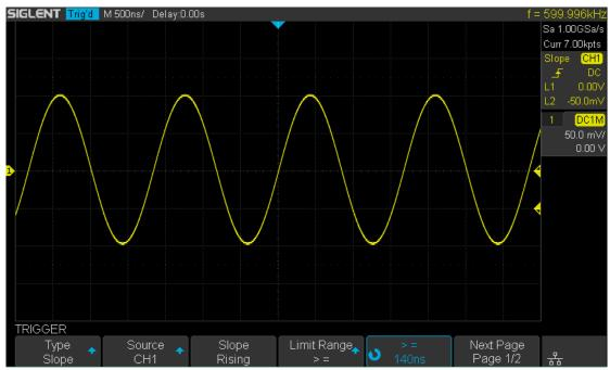
Figure 31 Slope Trigger
