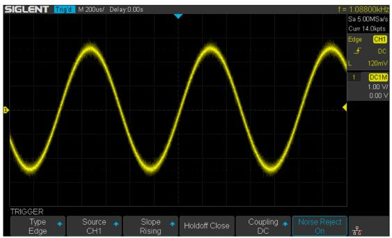
Figure 29 Turn on the Noise Reject
