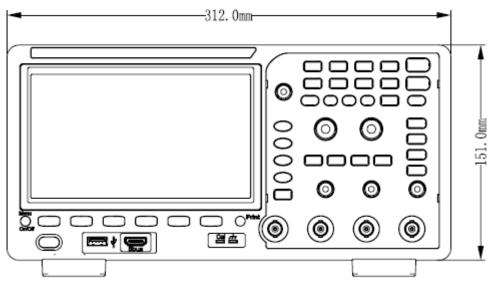
Figure 3 Front View (4-channel scope)
