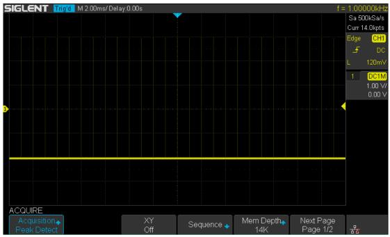
Figure 23 Pulse With 0.1% Duty, Peak Detect Mode
