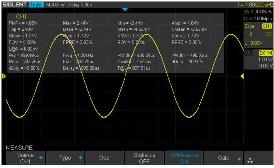
Figure 92 All Parameters Measurement
