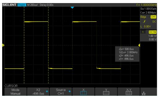
Figure 85 Measure Pulse Width
