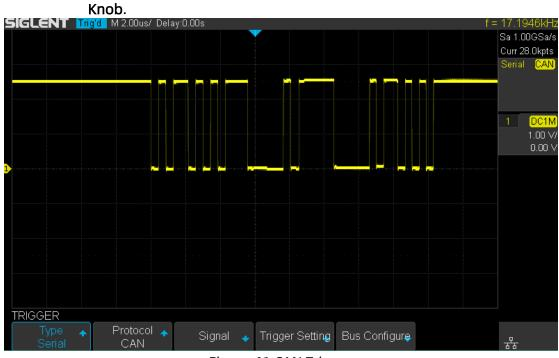
Figure 61 CAN Trigger
