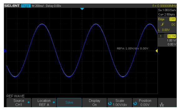
Figure 69 Reference Waveform
