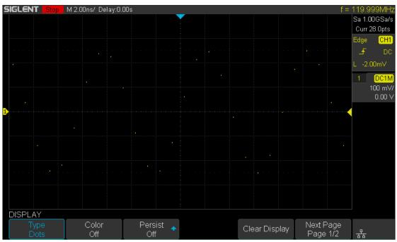
Figure 18 Display Type Set to Dots
