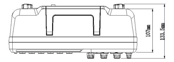
Figure 2 Top View (2-channel scope)
