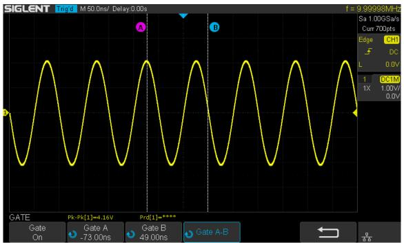
Figure 93 Gate Measurement
