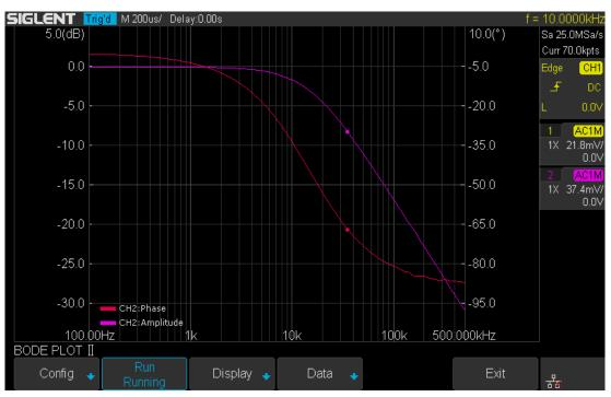
Figure 145 Bode Plot Sweep Curve
