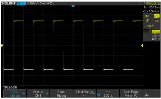
Figure 36 Interval Trigger
