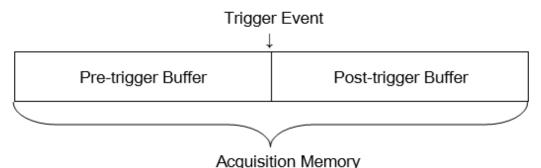
Trigger setting should be based on the features of the input signal, thus you need to have some knowledge of the signal under test to quickly capture the desired waveform.
