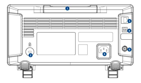
Figure 13 SDS1000X-U Scope Rear panel Overview
