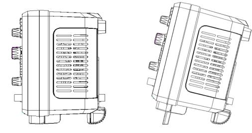
Figure 5 Adjust the Supporting Legs
