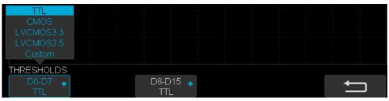
Figure 105 THRESHOLDS Function Menu
