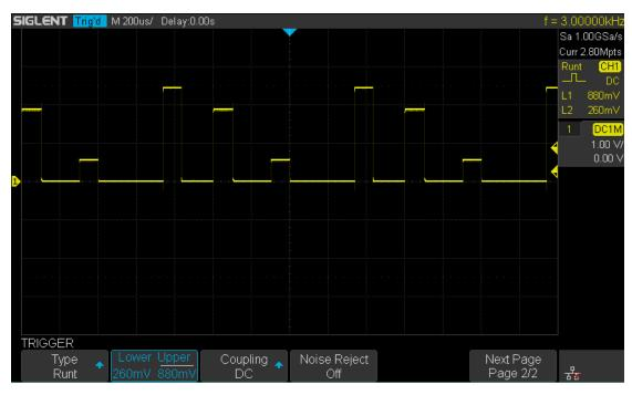
Figure 39 Runt Trigger
