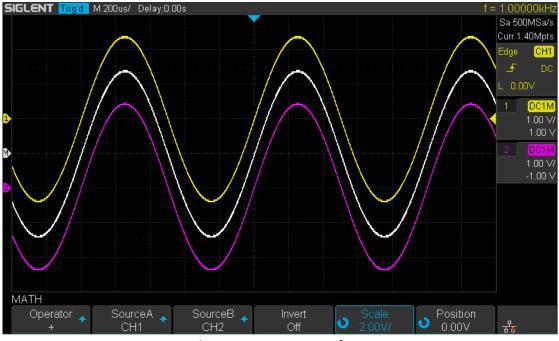
Figure 70 C1+C2 Waveform
