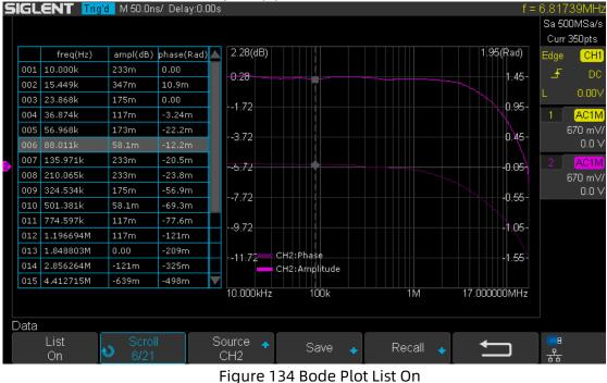
2) Press **Save** softkey (**Recall** softkey) to enable the bode plot save (recall) function. See the chapter "Save and Recall" for details.
