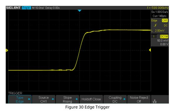
Holdoff, coupling and noise reject can be set in edge trigger, see the sections "Trigger Holdoff", "Trigger Coupling" and "Noise Rejection" for details.
