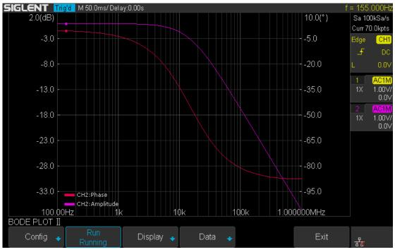
Figure 140 Bode Plot Sweep Curve
