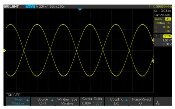
Figure 35 Relative Window Trigger
