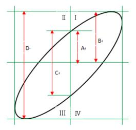
According to  $\sin\theta = A/B$  or C/D (wherein,  $\theta$  is the phase deviation angle between the two channels and the definitions of A, B, C and D are as shown in the figure above), the phase deviation angle is obtained, that is:  $\theta = \pm \arcsin(A/B) \operatorname{or} \pm \arcsin(C/D)$
