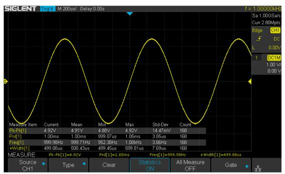
Figure 91 Added the Measurement
