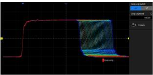
Segmented memory collection will store the waveform into multiple memory segments (up to 80,000) and each segment will store a triggered waveform as well the dead time information. The interval between segments can be as small as 2  $\mu$ s. All of the segments can be played back using the History function.
