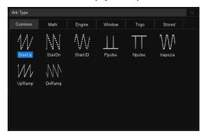
The USB waveform generator can output waveforms with up to 25 MHz frequency and ±3 V amplitude. Six basic waveforms together with multiple types of predefined waveforms and as user-defined arbitrary waveforms are supported.
