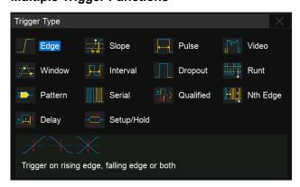
Edge, Slope, Pulse width, Video, Window, Runt, Interval, Dropout, Pattern, Qualified, Nth edge, Delay, Setup/Hold time, and Serial trigger.
