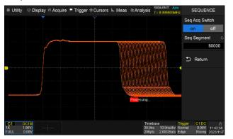
Segmented memory collection will store the waveform into multiple memory segments (up to 80,000) and each segment will store a triggered waveform as well the dead time information. The interval between segments can be as small as 2  $\mu$ s. All of the segments can be played back using the History function.
